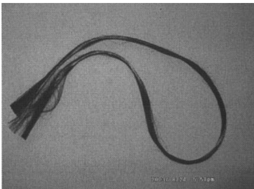
Figure 2 Optical graph of the recycled carbon fibers.
